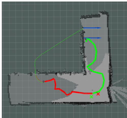
Fig. 5. Real-world exploration with two UGVs. Robot starting positions are indicated with an 'X' and the paths taken are shown with red and green lines, respectively.
