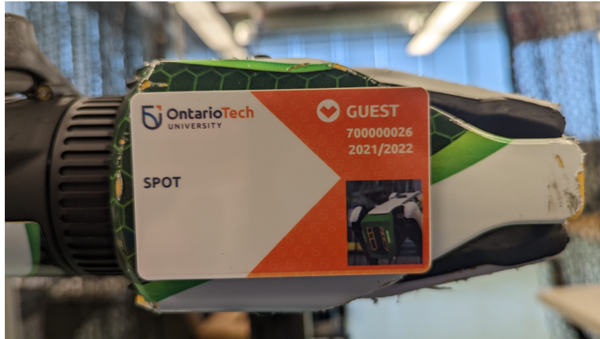
Fig. 7. Spot's access card attached to the underside of Spot's gripper.
