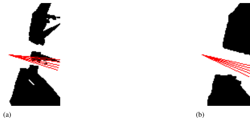
Fig. 5. The local grid and inspection lines that were used to determine the state of the elevator door. (a) With the elevator door closed. (b) With the elevator door open.
