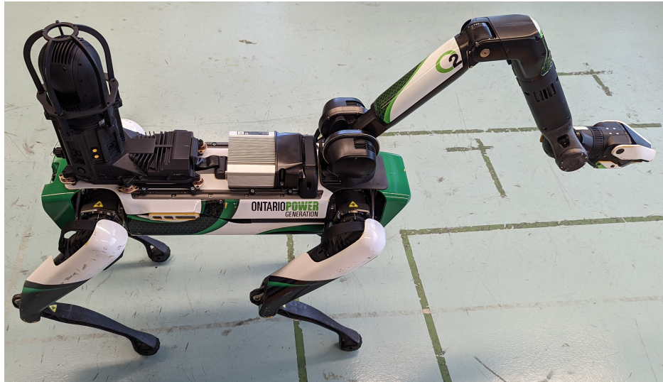
Fig. 1. The Spot robot used in this work equipped with the Spot Core computer payload and arm.
