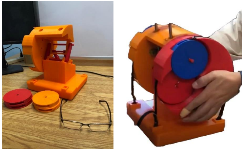
Figure. 2. Scaled up model of the four-bar driven knee model. Left: opened model to reveal mechanism. Right: drivable model with cables attached.
