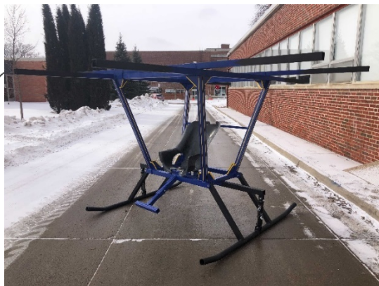
Figure 5: Albatross structure assembled
