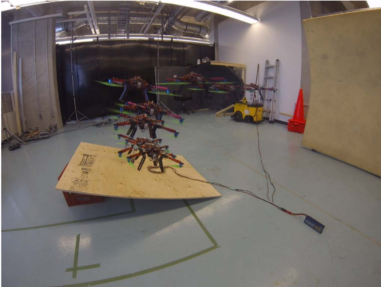
Fig. 8. An action-sequence of the OmniCopter landing on an inclined surface (20 degrees incline).
