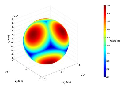
Fig. 5. Required applied wheel normal force for different directions of maximum sphere torque.
