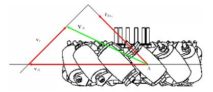
Fig. 4. Schematic of Mecanum wheel velocity vectors.
