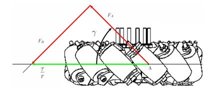
Fig. 3. Mecanum wheel roller forces.
