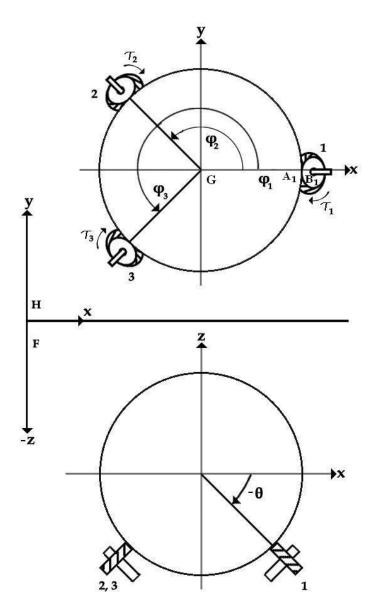
Fig. 2. Configuration of three driven wheels for Atlas.
