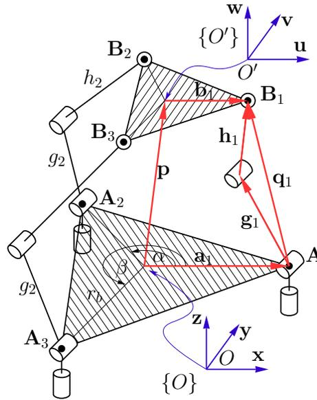
Fig. 4. 3-RRRS redundantly actuated parallel manipulator architecture, as denoted in [6].
