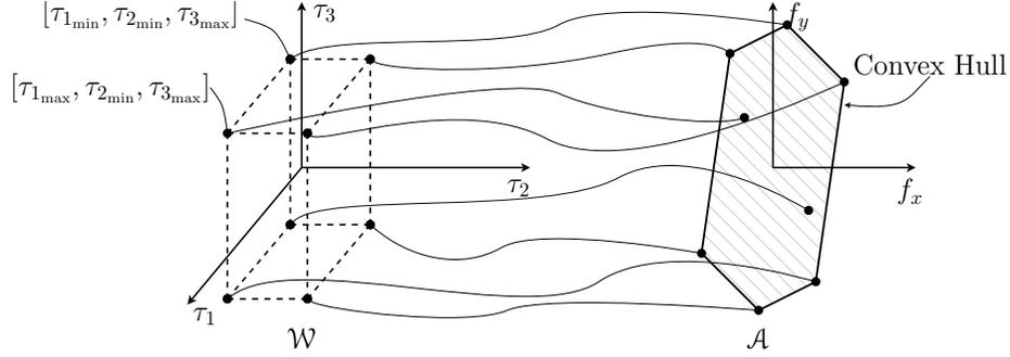
Fig. 2. Actuator Force Workspace (left) formed from the torque limits of three actuators ( $\tau_1, \tau_2, \tau_3$ ) mapped to form the Available Wrench Set (right) using the Jacobian matrix transformation [7].
