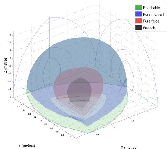
Fig. 6.  $\mathcal{J}_{HE}$  wrench workspaces showing pure force, pure moment, wrench, and reachable workspaces.
