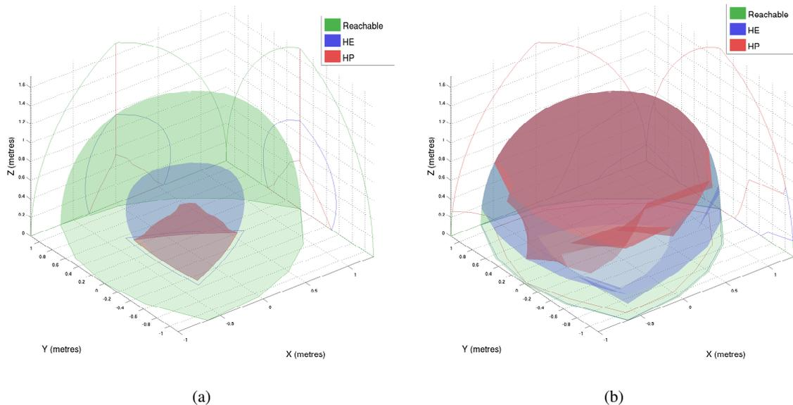
Fig. 5. Comparison of pure force (a) and pure moment (b) workspaces for the  $\mathcal{T}_{HP}$  and  $\mathcal{T}_{HE}$  wrench capability techniques.
