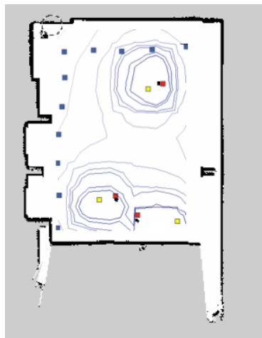
Fig. 6b. Radiation Map Generated by Radbot for Three-Source Exposure Scenario Test
