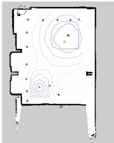
Fig. 4b. Radiation Map Generated by Radbot for Two-Source Exposure Scenario Test
