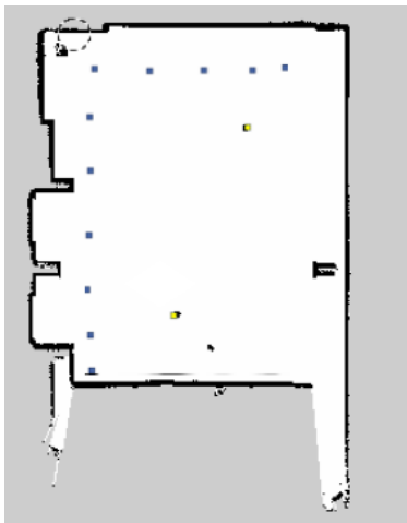
Fig. 4a. Locations Where Radiation Samples Were Collected and Used to Generate Map for the Two-Source Exposure Scenario Test
