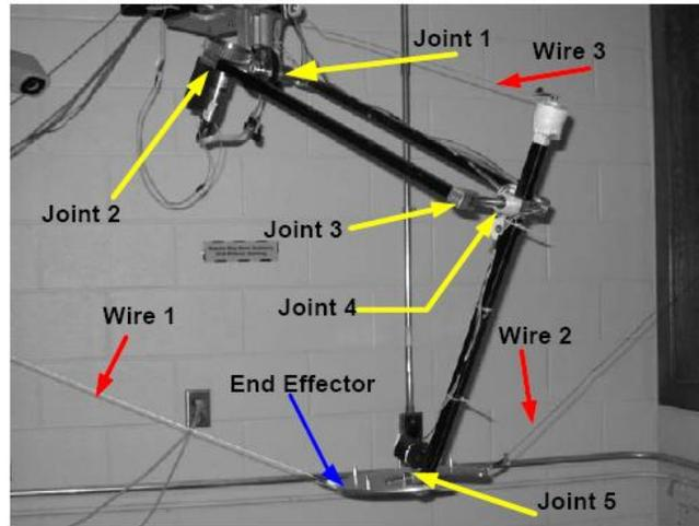
**Figure 1.** Wire-actuated parallel robot manipulator.
