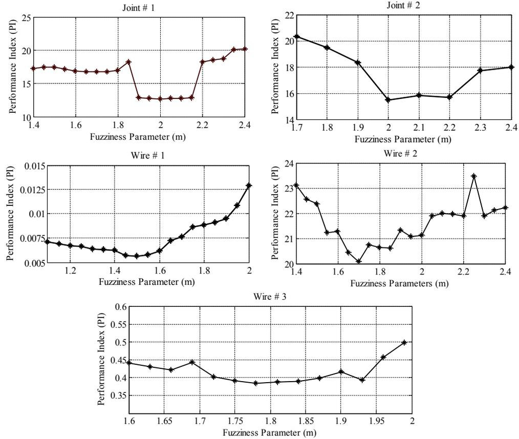
**Figure 4.** Performance index variation with the fuzziness parameter  $m$  for actuated joints/wires.
