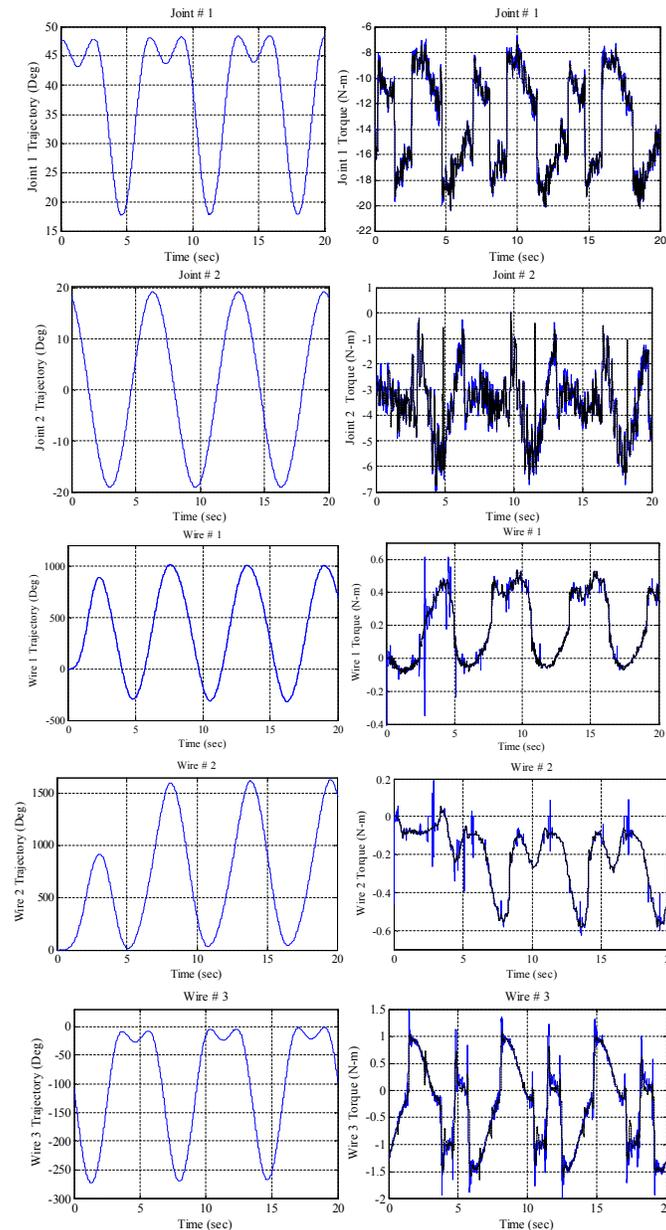
**Figure 6:** Comparison of the actuated joint/wire torque computed by fuzzy model (dotted line) with the measured joint/wire torque (solid line) for the sinusoidal and periodic trajectories.
