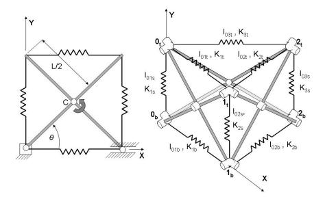
Figure 1: Planar (left) and spatial (right) tensegrity mechanisms.
