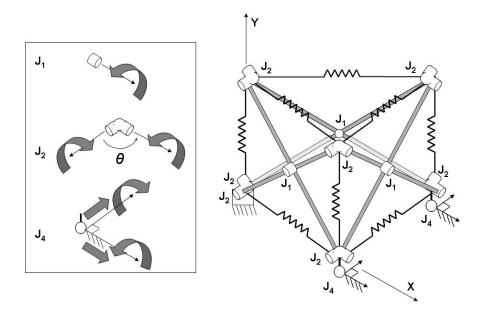
Figure 2: Spatial 1-DOF tensegrity mechanism and associated joints.
