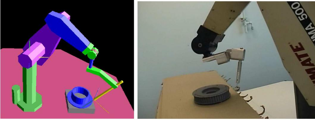
Figure 1: Arc-welding task with the PUMA 560 manipulator
