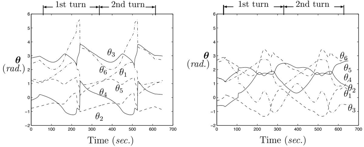
Figure 3: Joint position with respect to time for the augmented approach (left) and projected approach (right)
