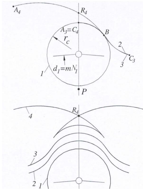
Fig. 2 Conjugate Tooth Profiles of Gearsets 1-2, 3-2 and 4-2 with  $N_1=N_3=N_4=11$ ,  $N_2=12$ ,  $x = 0.2$  and  $r_c^* = 1$
