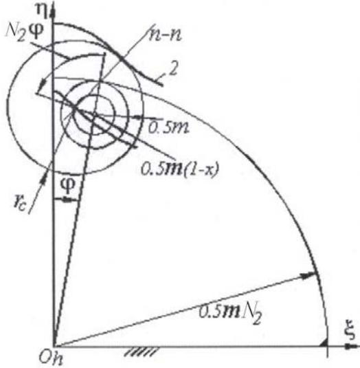
Fig. 2 Generating Tooth Profile of Epicycloidal Gear
