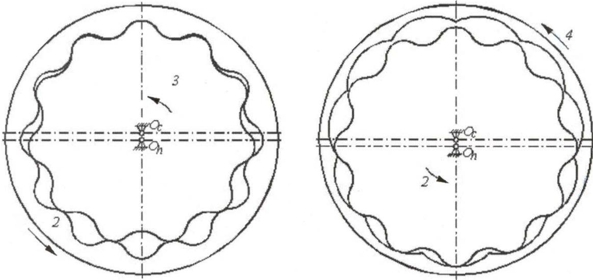
Fig. 6 Two Gearsets with  $m = 5$  mm,  $N_1 = 11$ ,  $N_3 \equiv N_4 = 12$ ,  $x = 0.2$  and  $r_c^* = 1$
