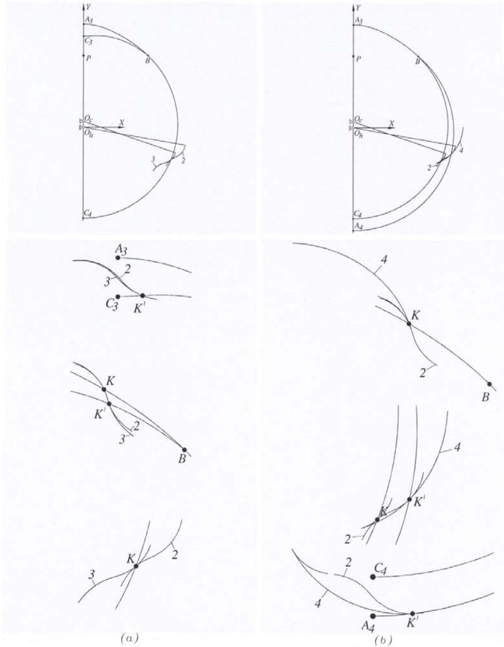
Fig. 4 Lines of Contact of Two Hypocycloidal Gearsets with  $m = 5$  mm,  $N_1 = 11$ ,  $x = 0.2$  and  $r_c^* = 1$
